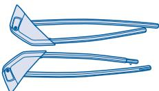
Insert slotted leg post through the frame of the seat, with logo facing out and the numbered leg on the side with window. Repeat with other leg. Make sure to squeeze button to choose one of the other height options.
